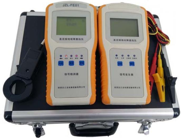
FST-JD200 not only can provide a solution on accurately testing the faults of the indirect-grounding of the direct current system, non-metal grounding, loop grounding, simultaneous grounding of the anode and cathode, balanced grounding of the anode and cathode and multi-point grounding; it also can accurately display the system voltage, voltage to ground and grounding resistance value. It truly eradicates the fear of trouble in the rear for the operating and testing personnel.
